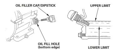
Oil is added to the engine by removing the oil cap and adding oil at this point. After filling the crankcase to the proper level, be sure you properly tighten the oil fill cap.
