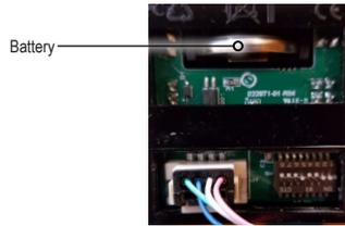
Replace the battery having the POSITIVE (+) side down. Ensure the battery is secured between the battery connections.
