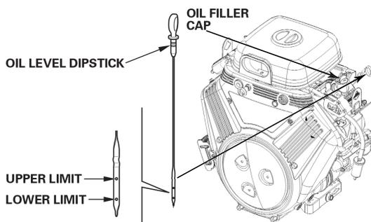
Oil is added to the engine by removing the oil cap and adding oil at this point. After filling the crankcase to the proper level, be sure you properly tighten the oil fill cap.
