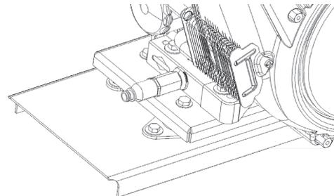
1. Start the engine and warm it up, stop the engine and remove the spark plug wire to prevent it from accidentally being started.
