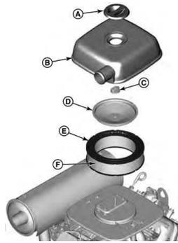
You can use pressurized air (not to exceed 30 psi) to clean the filter. Always blow the compressed air from inside to the outside.
