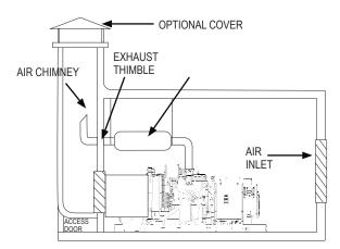
The muffler can be installed either inside or outside the shelter. Installing inside the shelter will increase the overall temperature and may require a larger shelter or additional air flow to prevent equipment overheating. In some cases, the muffler may require appropriate insulation to prevent radiant heat from affecting the equipment inside the shelter.
